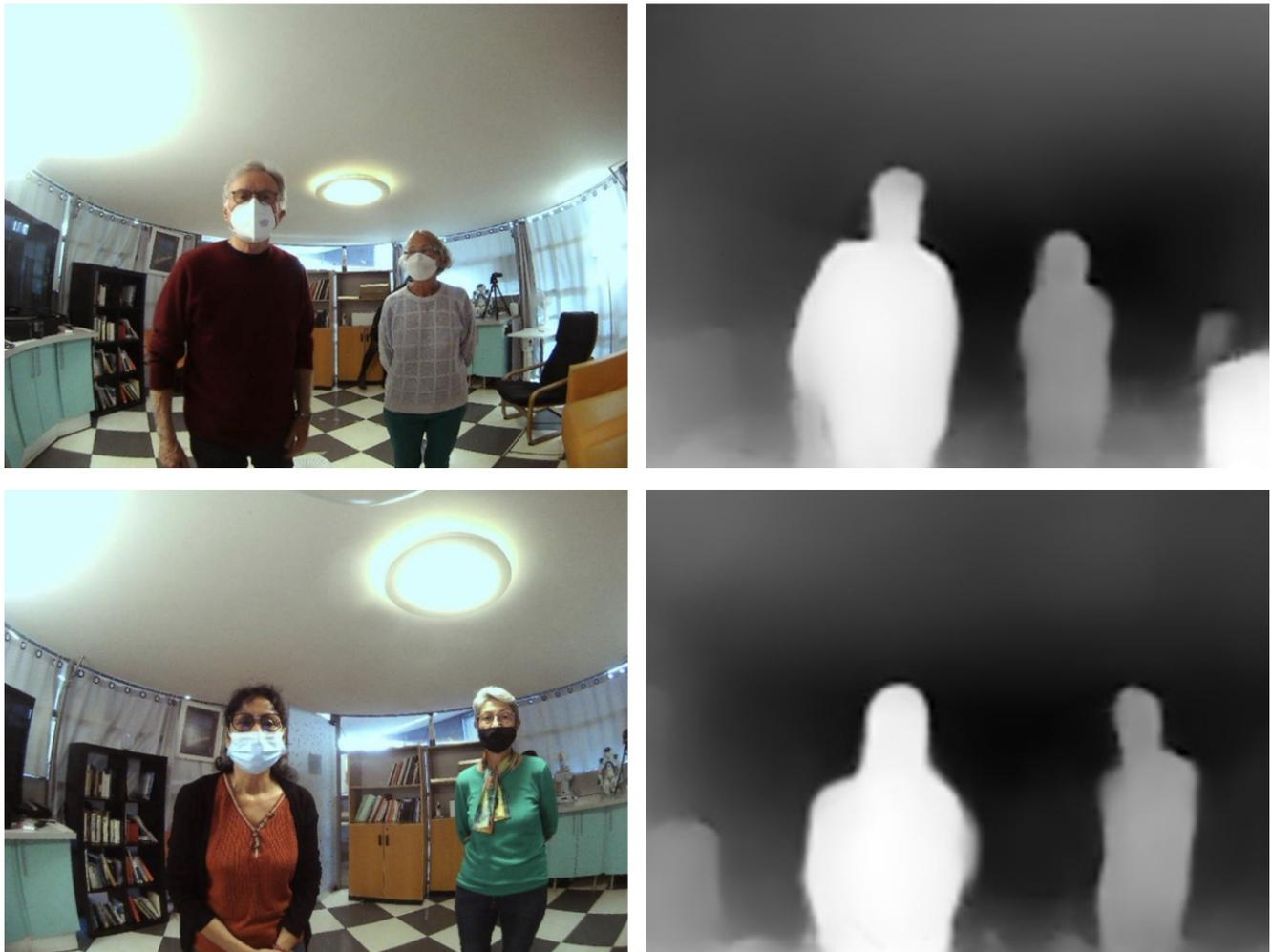
Figure 2.4: The monocular depth estimation model running on the rectified images of the front fisheye camera of ARI.
