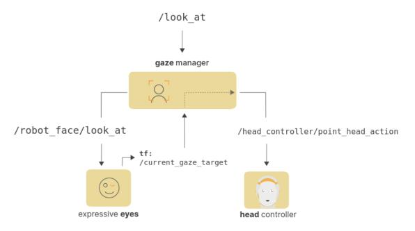
Figure 3.8: Gaze Manager that controls both eyes and head position.
