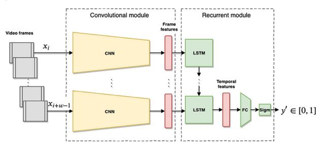
Figure 4.4: Overview of the model proposed in . The input is a video stream of interactions between the robot and humans collected in w size intervals. The frames xi are passed through the pre-trained CNN (ResNet) producing a per-frame feature vector which is then passed sequentially to the LSTM network. After w steps the LSTM produces a temporal feature vector which is passed to a FC layer with sigmoid activation to produce an engagement value y for the temporal window.
