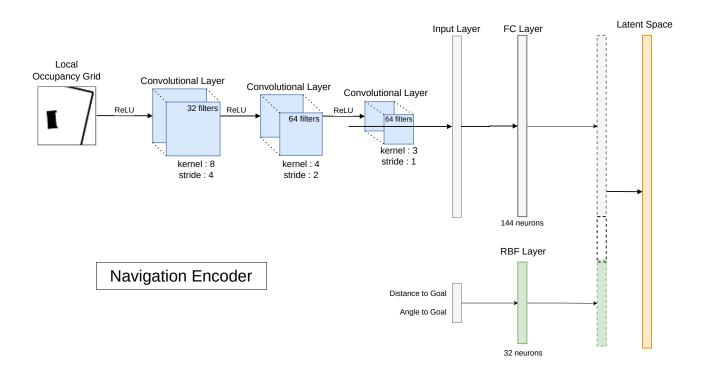
Figure 3.5: Navigation Encoder: The encoder takes as input the state and computes a latent representation. The encoded representation is then given to the actor and critic network to compute respectively the policy and the Q-value. The robot-centric occupancy grid is encoded with a CNN. The polar coordinates of the goal are encoded with a Radial Basis Function layer [2].
