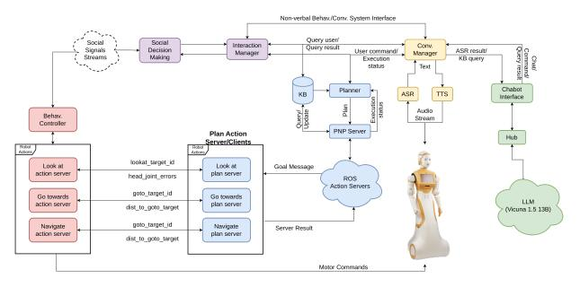
Figure 2.2: System architecture for the Robot Non-verbal Behaviour System; and the interface between the non-verbal behaviour manager, the task planner, and the conversational system. The non-verbal behaviour manager (in purple) the high-level planning framework (in blue), the conversation manager interface (in yellow) and the conversational system on the right (in green) with the robot non-verbal behaviour manager components (in red) on the left.
