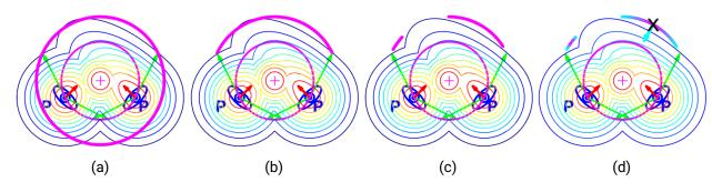
Figure 3.4: Estimation of the approaching pose. (a) The approaching area is the thick outer magenta circle. (b) Filtered approaching areas by human FOV, and (c) the social space  $F_{soc}$ . (d) The final approaching pose (black x) is the central point of one of the remaining approaching area segments. Figures adapted from [31].
