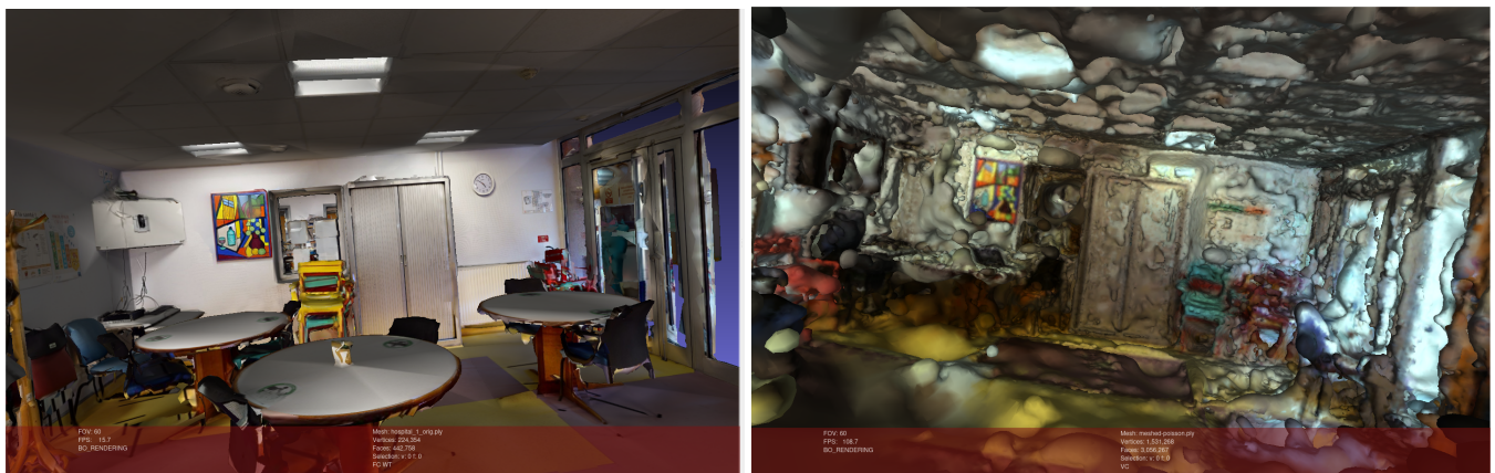
Figure 1.10: Dense reconstruction of the first floor of the Broca hospital. Snapshots of the same region in the Broca hospital are presented, with the left image showing the results of Matterport 3D scanning and the right image displaying the SfM reconstruction from ARI images. The dense model derived from Matterport is complete and less noisy than the reconstruction obtained from ARI images.
