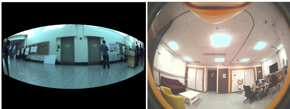
Figure 2.2: Left: attempt to transform the central part of the panoramic image of Fig 2.1 into the fisheye geometry. Right: image captured from ARI's front fisheye camera.
