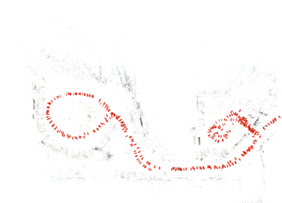
(b) COLMAP map reconstruction created from the blur and distance filtered data. The data filtering process is described in 4.0.2
