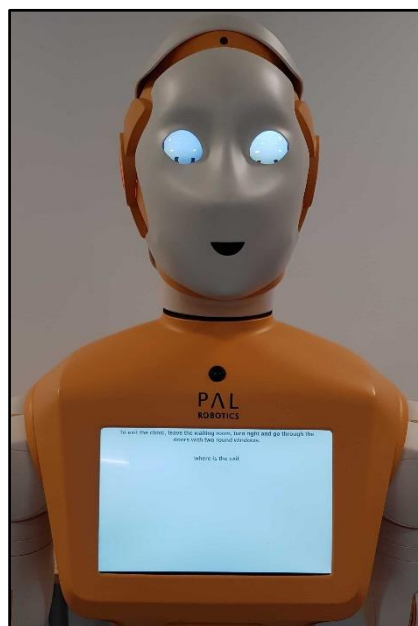
Figure 1 ARI Display Screen - TTS and ASR outputs
