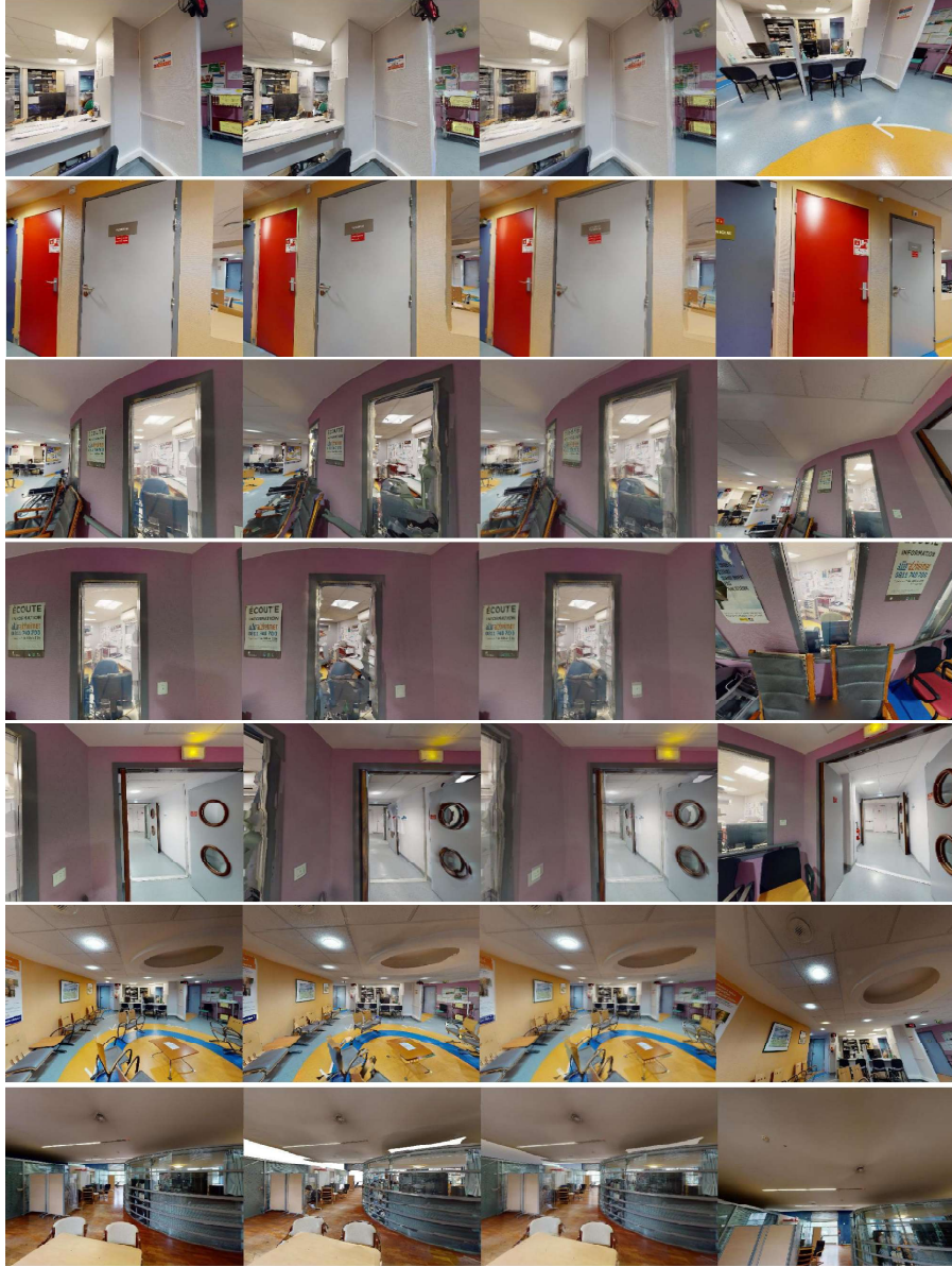
Figure 10: Columns from left to right: Well localised query images, projected mesh from estimated pose, blend of query and mesh projection, database image used for relative pose estimation.
