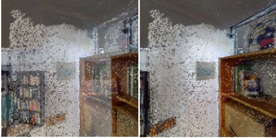
Figure 8: Blended mesh projection with a cutout of a panorama. The reference rotation (left) compared to our estimate (right).
