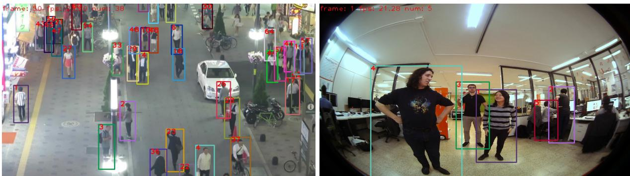
Figure 2: Example of tracking with FairMOT. Left: on the MOT16 dataset. Right: On an image sequence captured by ARI’s front fish-eye camera.
